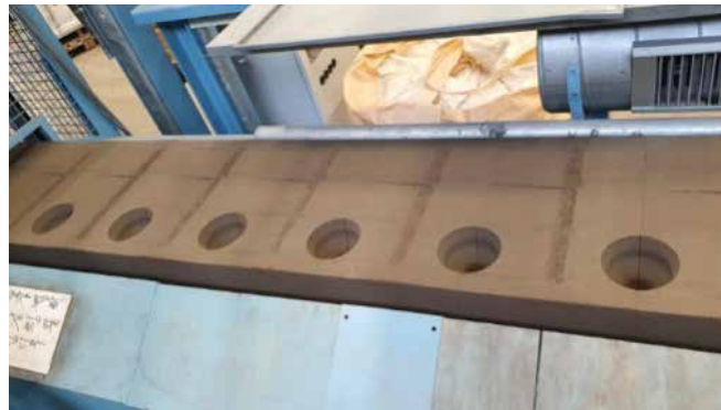
Figure 10 : Mould string ready for pouring.
