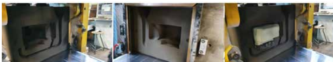
Figure 9 : Left: Pressure plate mould. Centre: Swing Plate mould. Right: Pressure plate mould with core.
