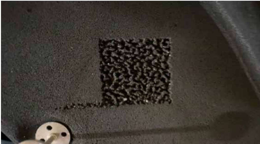
Figure 10: %100 Readable CDOT code engraved in the sand mold with 60W fiber laser and 110mm lens in the production
