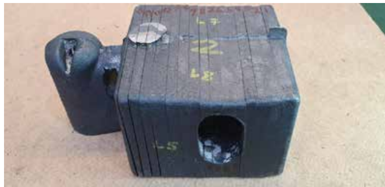
Figure 11 : Casting sliced for inspection.
