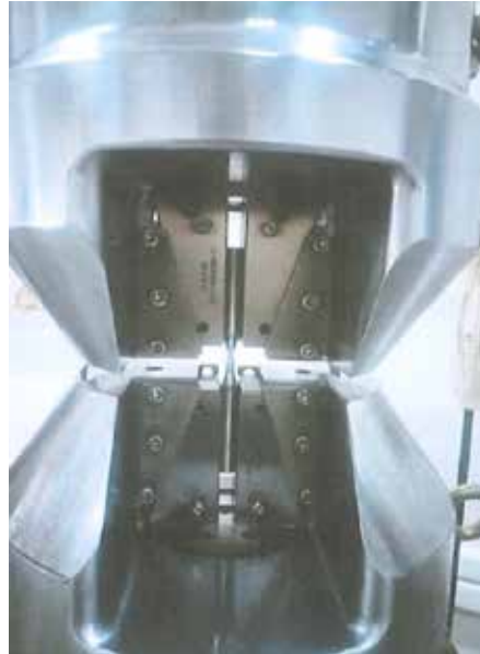
Figure 4: Test Configuration and Fatigue Limit Test Specimen [1]
