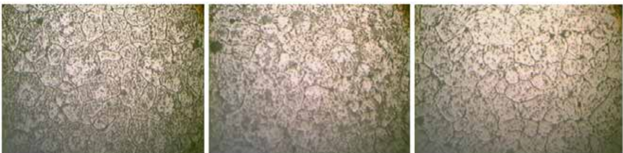
Figure 2: Microstructure of Specimen 1,2,3(with vibration) in Optical Microscope at 400x Magnification
