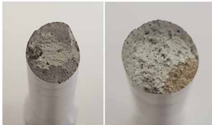
Figure 9: Fracture Surfaces of Specimen 3 and Specimen 6
