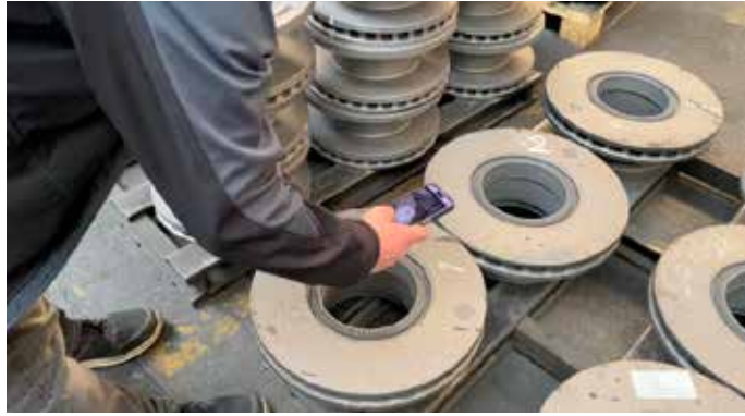
Figure 13: CDOT code reading on transferred CDOT code
