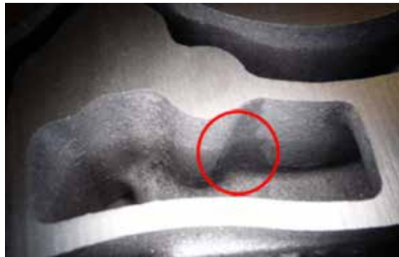
Figure 2 : Aluminum silicates mix, graphite coating with good thermal stability and additional “sintering phases” Arkopal®
