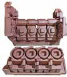
Figure 1: Coated core package, Image from HA Group
