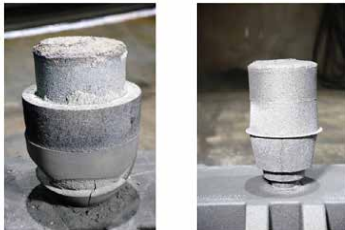
Figure 9: View of the breaking edge area after shake-out and fettling
