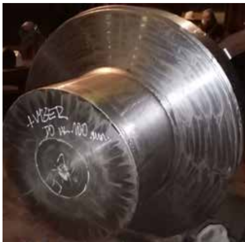
Fig 13a: Porosity in bottom hub
