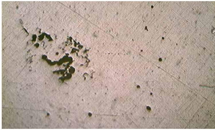
Figure 7: Intermetallic Compound in Chinese Script Morphology in Specimen 3
