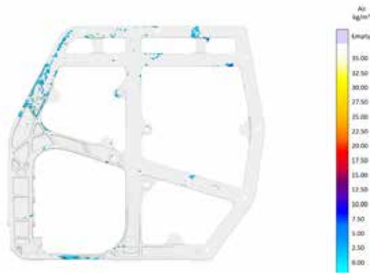
Figure 10: Air results of the part without air pockets with vacuum
