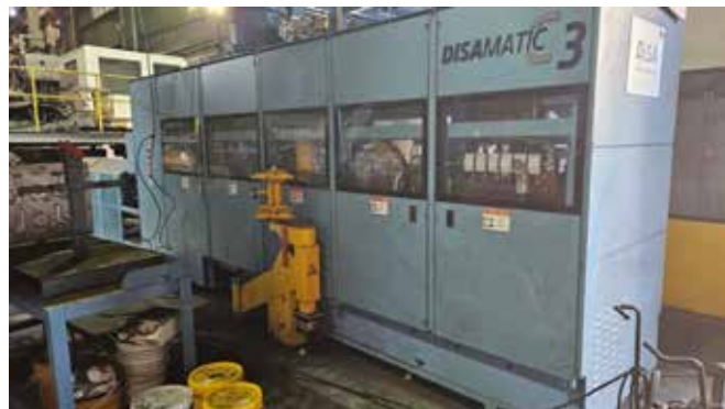
Figure 4 : DISAMATIC C-250 after producing 10,000,000 moulds.
