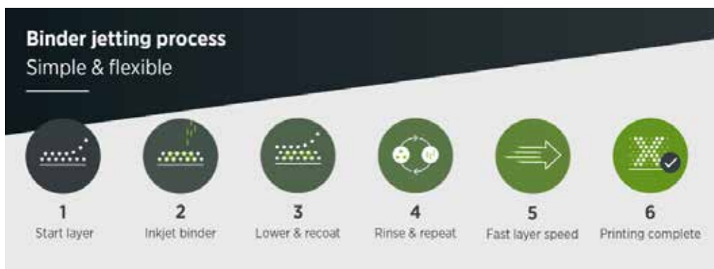
Figure 1: Binder jetting process
