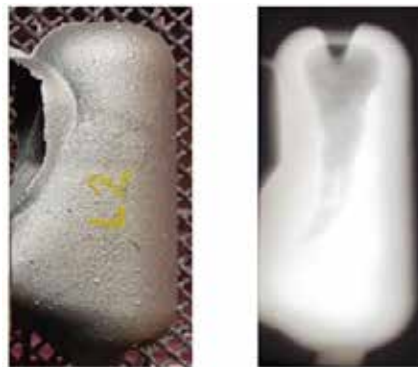
Figure 15 : X-ray of container corner casting feeder neck.
