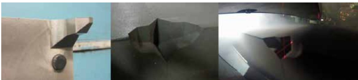
Figure 6 : Left: Reference blocks added to pattern plates. Centre: Reference impressions on the mould. Right: Lasers measuring in real time.
