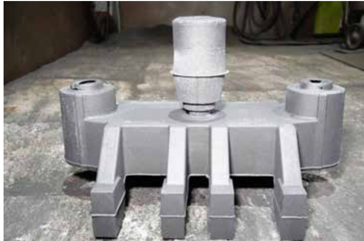
Figure 8: View of the casting part after fettling
